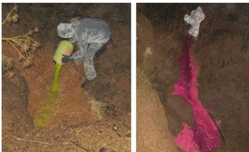
Fig. 5. Left: Uranine injection into the Argamasilla cave swallow-hole (IP1); Right: Sulforhodamine B injection into the IP2.
